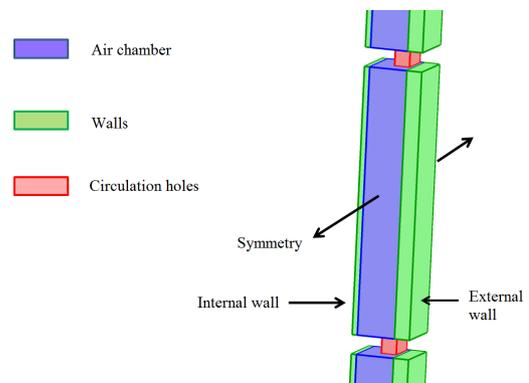
**Figure 3.** Geometric diagram of the simulation module.
