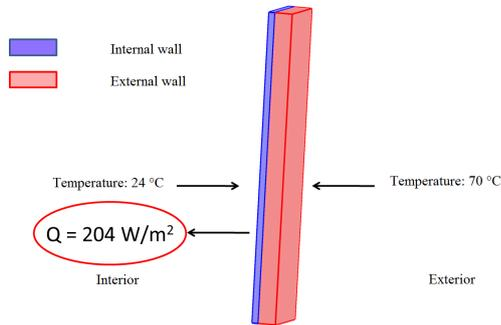
**Figure 4.** Simulation conditions and thermal energy for absence of cavity.
