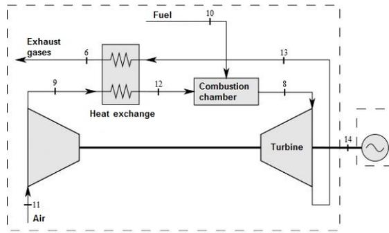
Figure 6. Control volume of the Brayton cycle [41].
