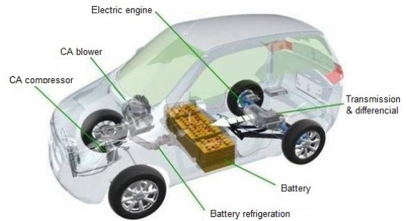
**Figure 1.** Basic components of an electric vehicle [7].
