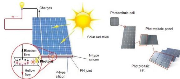
Figure 2. Operation of the PV panel [18].
