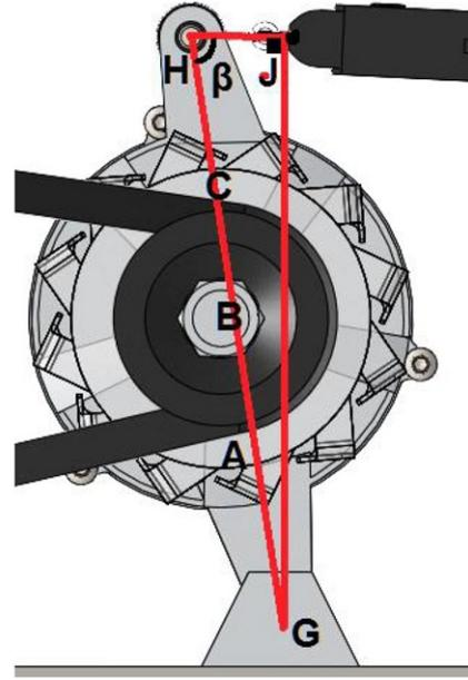
Figure 4. Tension system of the module band.
