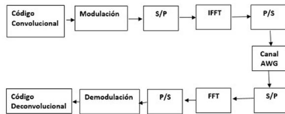
Figure 1. OFDM with convolution code.
