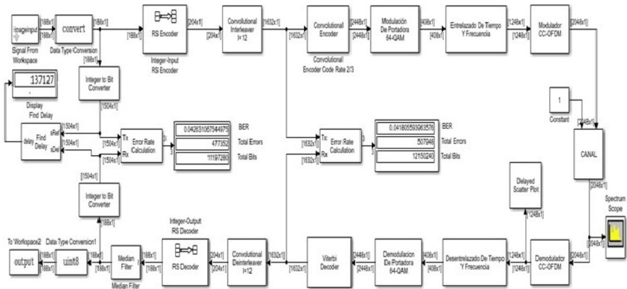
Figure 2. Block diagram of the ISDB-T standard with OFDM modulation, created in Matlab Simulink.
