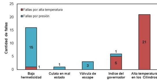
**Figure 6.** Most significant failures caused by injection pressure and temperature in the combustion chamber in 2018.
