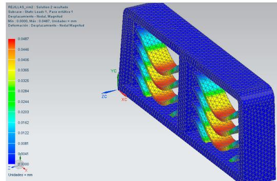
Figura 14. Graph of nodal displacement of the air conditioning grilles.
