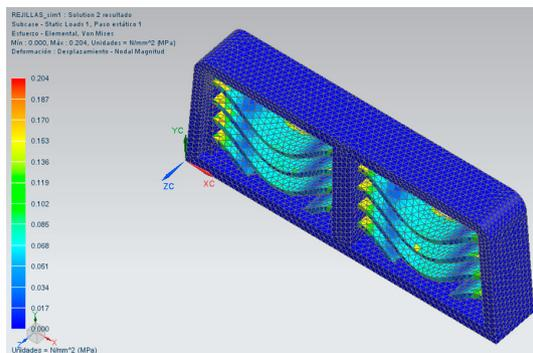
Figura 13. Graph of stresses generated on the air conditioning grilles.
