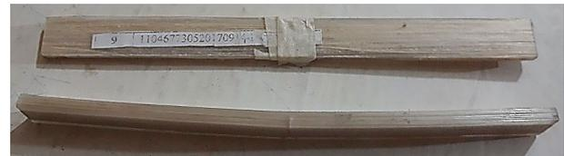
**Figure 8.** Test specimens of the composite material reinforced with abaca fibers.
