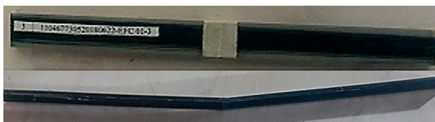
**Figura 10.** Test specimens of the composite material reinforced with cabuya fibers.
