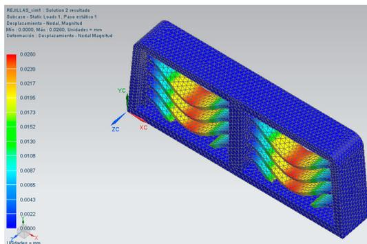
Figura 12. Graph of nodal displacement of the air conditioning grilles.
