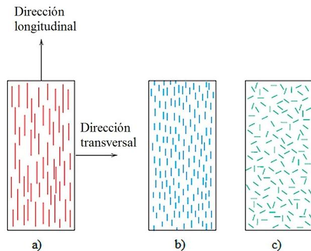
**Figura 1.** Possible orientations of the reinforcement in a composite material: a) continuous and aligned fibers, discontinuous and aligned fibers, and c) randomly oriented discontinuous fibers; taken from [11].
