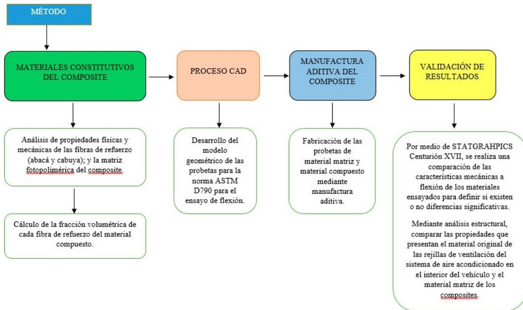
Figura 2. Steps for obtaining and validating the composite material.
