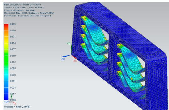
Figura 15. Graph of stresses generated on the air conditioning grilles.
