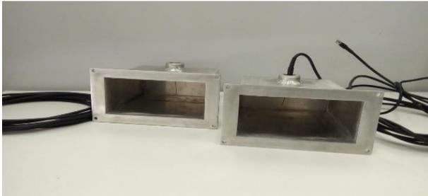
**Figure 4.** Aperture antennas utilized in MC measuring tests.
