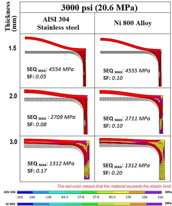
Constant temperature = 160 °C and internal pressure 3000 psi (20.6 MPa)
