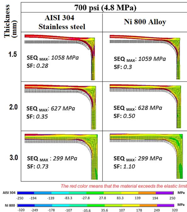
Constant temperature = 160 °C and internal pressure 700 psi (4.8 MPa).
