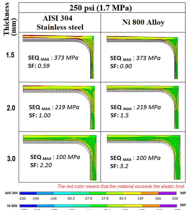
Constant temperature = 160 °C and internal pressure 250 psi (1.7 MPa)
