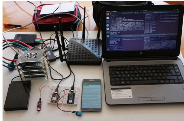
**Figure 4.** Setup for tests: from left to right it is observed a cluster of 3 Raspberry Pi running all services on Docker; an ESP8266 monitoring the level of noise with a KY038; an MKR1010 monitoring ambient temperature with an DHT11; an N9005 injecting random messages, and a laptop monitoring all services.
