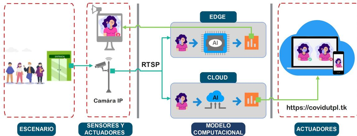
Figure 2. System architecture
