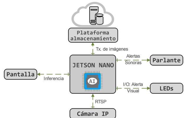
**Figure 4.** Architecture of the Edge computational model
