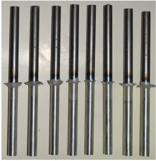
**Figure 6.** Welded test tubes, where it may be observed different configurations of the flash on the aluminum shaft
