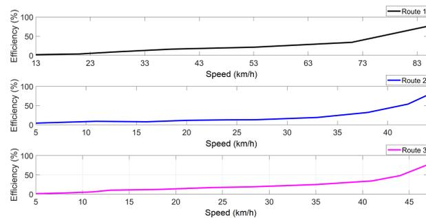
**Figure 6.** Efficiency of regenerative braking at specific speeds
