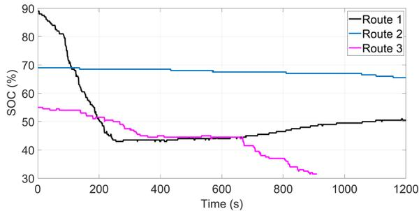
**Figure 4.** Behavior of SOC with respect to recovered energy
