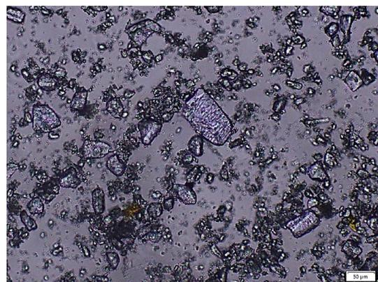
**Figure 9.** Lactose particles after 48 h of grinding
