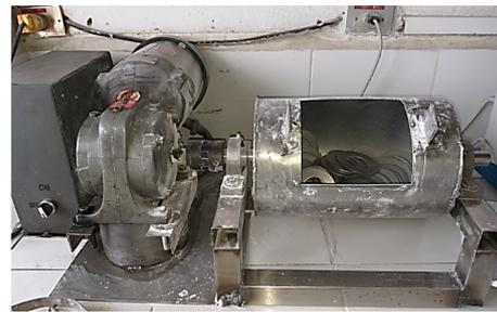
**Figure 4.** Horizontal rotating mill
