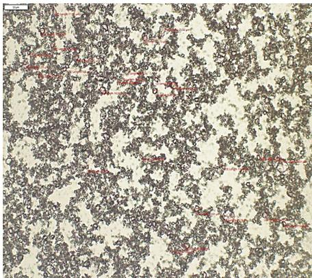
**Figure 12.** Lactose particles grinded for 5 h – Scale 50 μm
