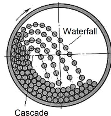
Figure 1. Movement of the load in a ball mill [5]
