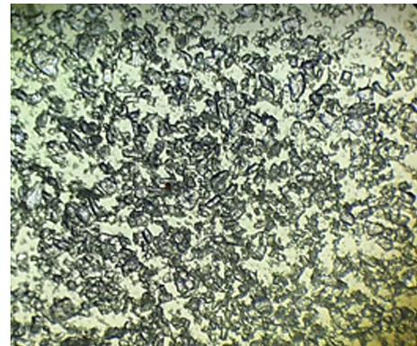
**Figure 13.** Lactose particles grinded for 1 h – Scale 100 μm
