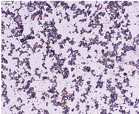
**Figure 11.** Lactose particles grinded for 1 h – Scale 100 μm
