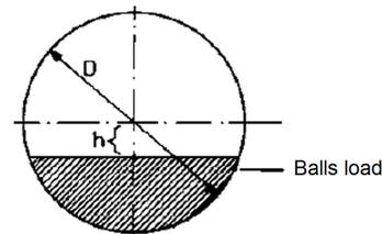
**Figure 10.** Filling of grinding material [1]
