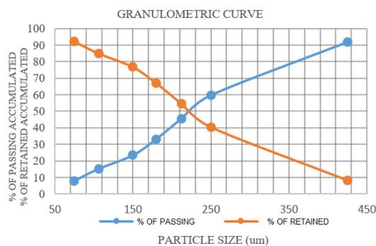
**Figure 7.** Percentage of passing accumulated and retained accumulated vs. particle size
