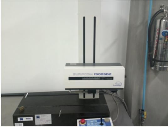
**Figure 4.** CARL ZEISS rugosimeter model SURFCOM 1500SD2.
