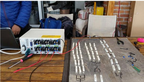
**Figure 2.** HIOKI PW 3337-03 equipment and load resistors
