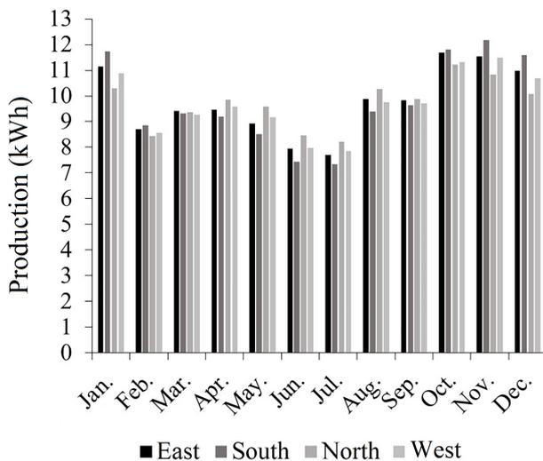
**Figure 5.** Estimated monthly production by simulation in SAM
