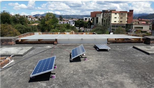
**Figure 1.** Monocrystalline solar panels with different inclinations
