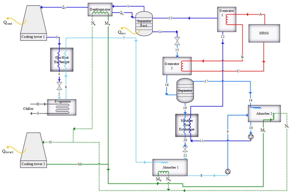
Figure 3. Double stage absorption equipment and auxiliary systems.
