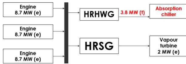
Figure 1. Powered cogeneration plant studied.
