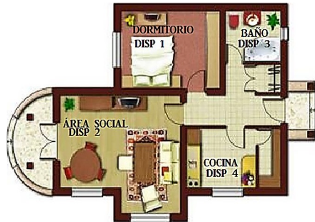
Figure 9. Distribution of measuring devices in a standard household.
