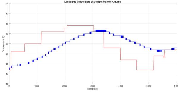
Figure 6. Real-time reading of temperature (ON/OFF).
