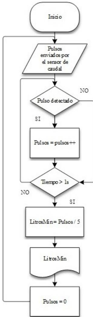
Figure 2. Calibration of the flow sensor.
