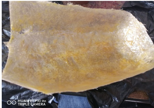
Figure 8. Rearview mirror with a cabuya fiber matrix.
