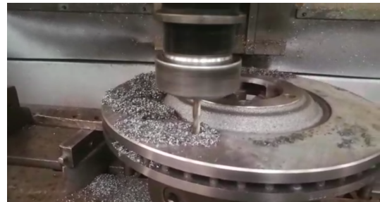
Figure 5. Drilling of the brake disc
