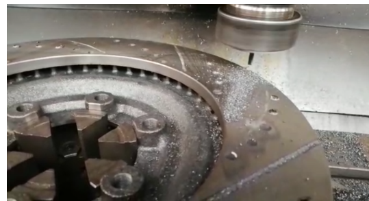
Figure 6. Grinding of ventilation slots
