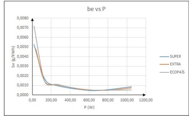
Figure 6. Curves of specific consumption vs. power
