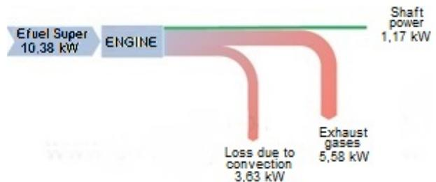
**Figure 9.** Sankey Diagram-Super Gasoline
