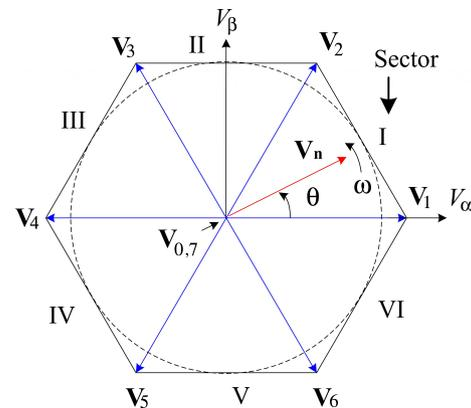
**Figure 3.** SVPWM modulation
