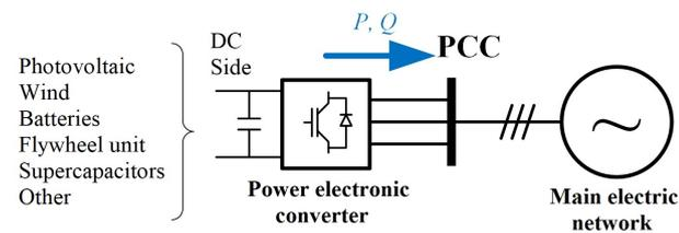
**Figure 1.** Power electronic converter connected to the grid
