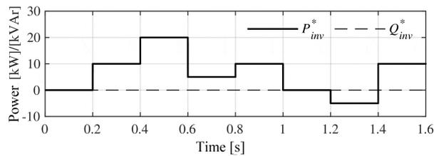
**Figure 13.** Power set-point signals applied to the converter
