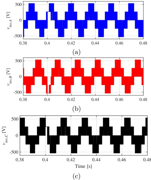
**Figure 6.** Three-phase generated at the inverter terminals
