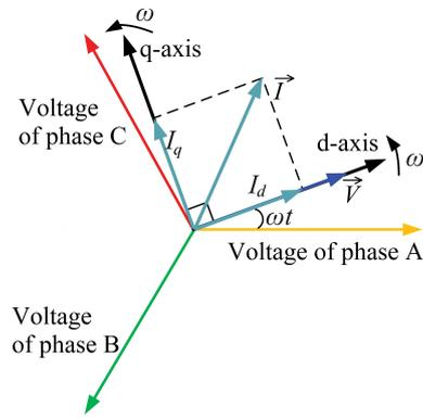
Figure 4.  $d - q$  coordinate system
