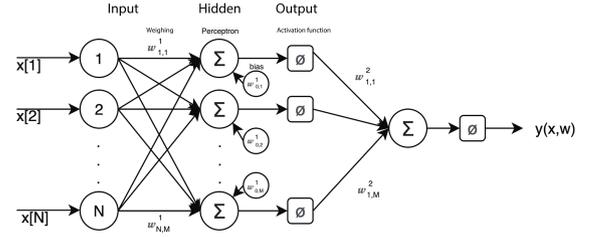
Figure 7. Structure of the proposed neural network.
