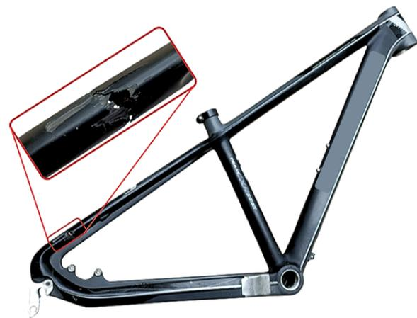
Figure 1. Failure in the upper chainstays
