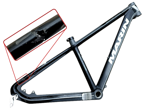
Figure 1. Failure in the upper chainstays
