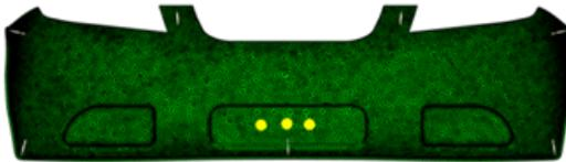
**Figure 6.** Design 3 (3 Resin Entry Points, 7 Vacuum Points)
