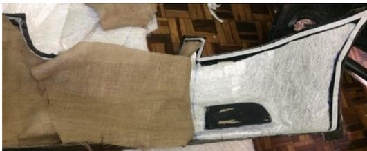
**Figure 12.** Arrangement of Fiberglass and Cabuya Fibers on the Mold
