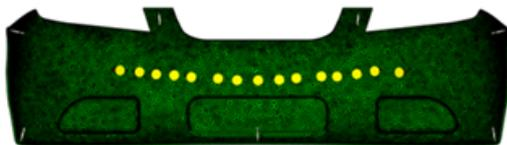
**Figure 8.** Design 5 (Multiple Resin Entry Points, 7 Vacuum Points)
