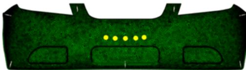
**Figure 7.** Design 4 (5 Resin Entry Points, 7 Vacuum Points)
