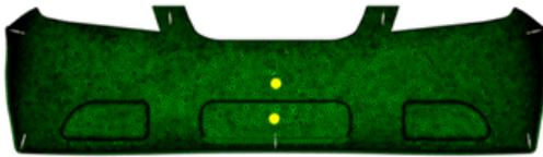
**Figure 5.** Design 2 (2 Resin Entry Points, 7 Vacuum Points)
