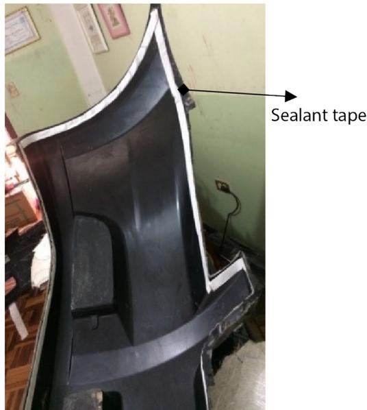
**Figure 11.** Placement of Sealant Tape on the Mold
