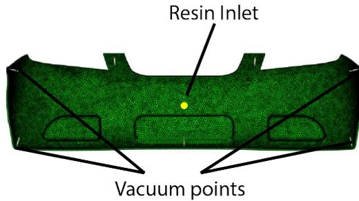
**Figure 4.** Design 1 (1 Resin Entry Point, 7 Vacuum Points)
