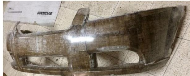
**Figure 19.** Side view of the bumper prototype obtained through VARTM
