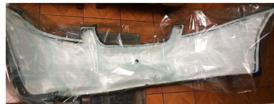
**Figure 15.** Vacuum bag used for the VARTM process
