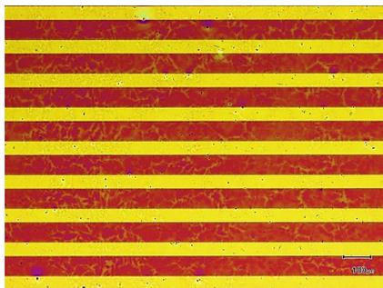
**Figure 3.** Photograph obtained by optical microscopy of a typical film of the DB-TTF and PS10k composite material in a 1:3 ratio; the angle between the polarizer and the analyzer is  $0^\circ$
