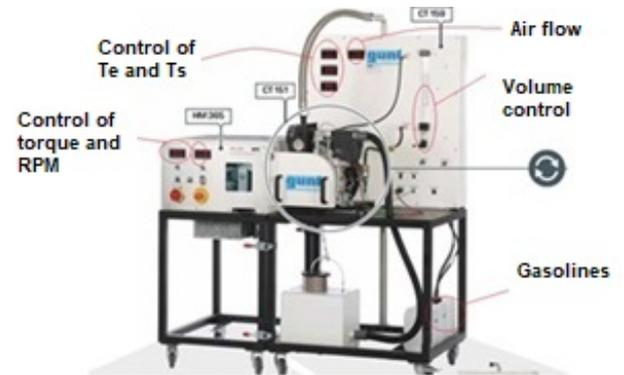
**Figura 4.** Experimental bench. Air-cooled gasoline engine with 1 cylinder, and HM 365 universal drive and brake unit
