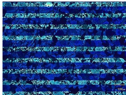
**Figure 4.** Photograph obtained by optical microscopy of a typical film of the DB-TTF and PS10k composite material in a 1:3 ratio; the angle between the polarizer and the analyzer is  $90^\circ$
