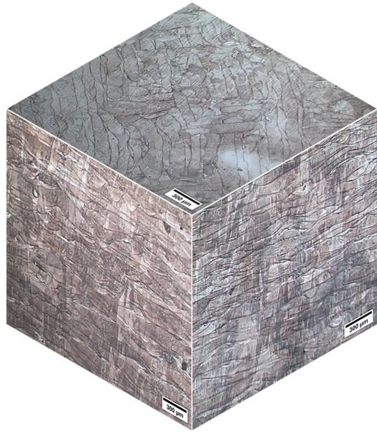
**Figure 4.** 3D assembly of optical micrographs of the 316 L stainless steel processed by LPBF.
