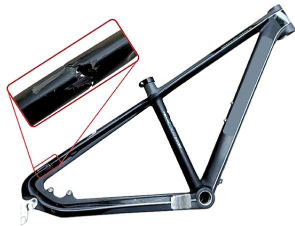
Figure 1. Failure in the upper chainstays
