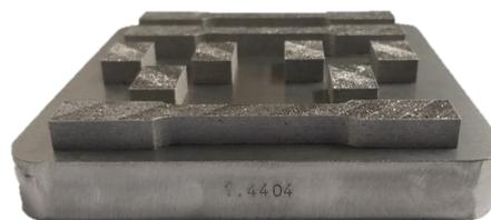
**Figure 2.** Additively manufactured samples for microstructure and mechanical evaluation. Base plate dimension: 100 x 100 x 16 mm.
