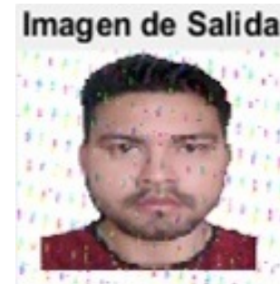
Figure 6. Output image after passing through site C with SNR=16 [dB] and OFDM modulation.
