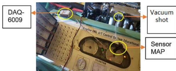
Figure 2. Connection of the MAP sensor.
