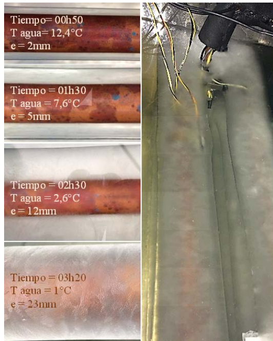
Figure 4. Thickness of ice at different time intervals. Practice 2.
