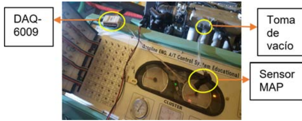
Figure 2. Connection of the MAP sensor.
