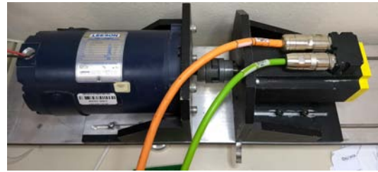
Figure 22. PMSM employed (left) and DC motor used as load (right).
