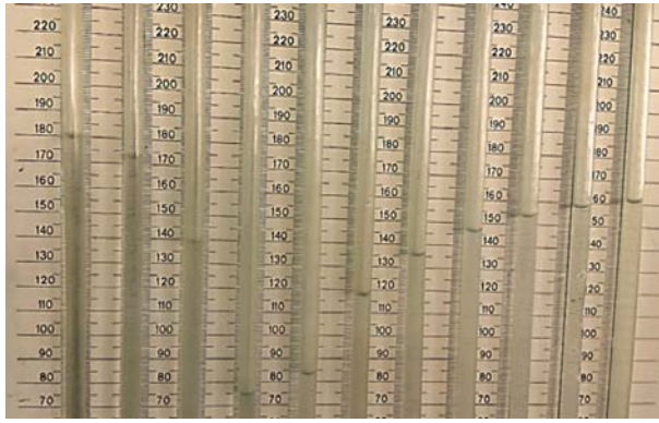
Figure 7. Piezometric heights for different levels of the water columns, corresponding to experiment 3.
