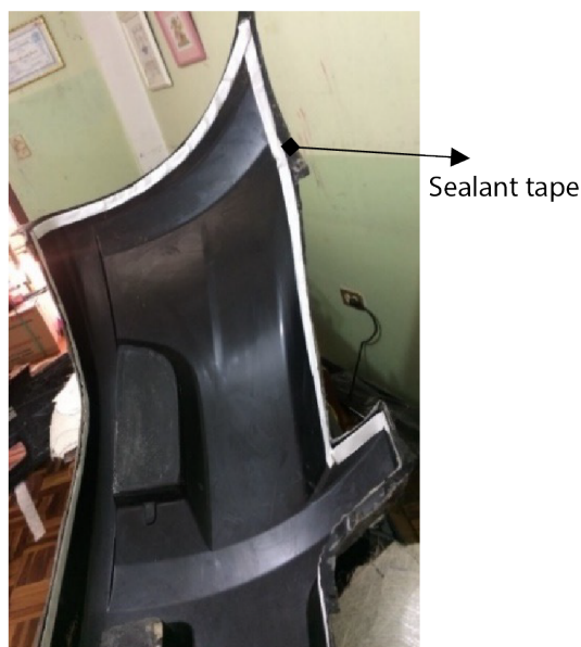
Figure 11. Placement of Sealant Tape on the Mold
