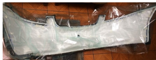
Figure 15. Vacuum bag used for the VARTM process
