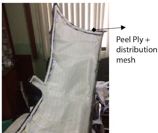
Figure 13. Peel Ply and distribution mesh over the fibers used as reinforcement.
