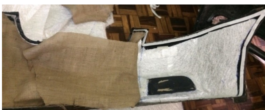
Figure 12. Arrangement of Fiberglass and Cabuya Fibers on the Mold
