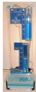
Figure 3. Coupled tank system
